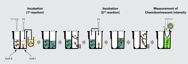
The sample together with diluent is pipetted in Cell I, while diluent is pipetted in Cell II.
